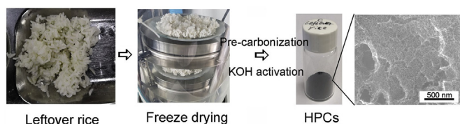
Scheme 1. Schematic illustration of the preparation process of the hierarchical porous carbons from leftover rice.
