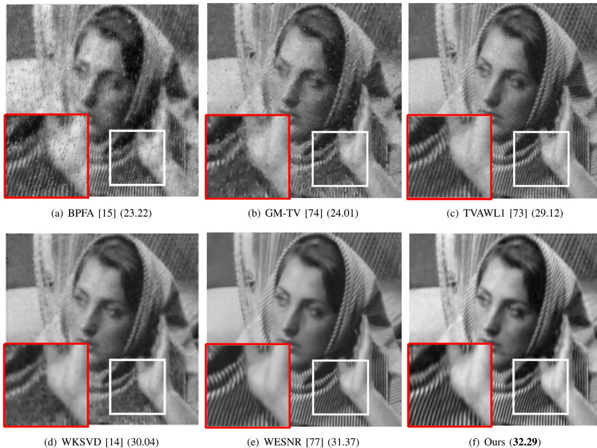
Fig. 6. Denoising results of different algorithms on Barbara image corrupted by mixed noise (standard deviation of Gaussian noise 10 and ratio of salt-and-pepper noise 10%). The PSNR results are reported in the parentheses.
