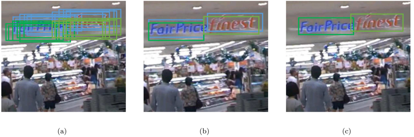
Fig. 4. The locality-aware NMS process. (a) The dense text boxes with different rows. (b) The dense text boxes are merged row by row. (c) The boxes are got through locality-aware NMS.
