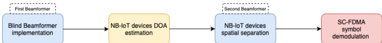
Figure 5.5: Block diagram with the steps needed at the LEO satellite to implement the proposed RSBA scheme to point device by device.
