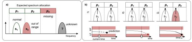
Fig. 3. Signal classification example (a) and anomaly prediction (b)
