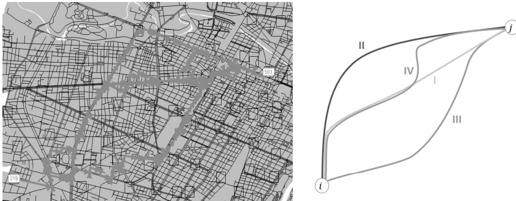
Figure 6 – Path set ( K_{ijr} ) for a certain Origin and Destination in the real network
