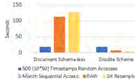
Fig. 1. Query execution time comparison for single vs multi-schema database.
