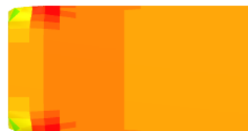
Figure 3.71: Pressure perturbations caused by a bad transition.
