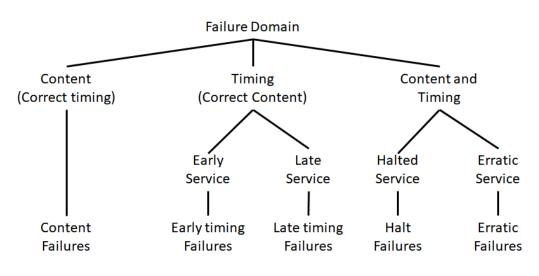
Fig. 2. Failure modes according to their domain
