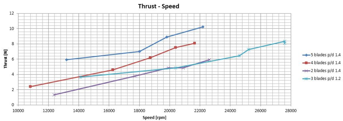
Figure 12 Thrust as a function of the rotor speed for various propellers configurations.
