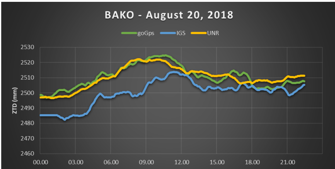
Figure 5.5. Same as Figure 5.3, but the date is 20 Aug 2018. The standard deviation and RMS of the difference between goGPS and IGS are 7.44 and -0.66, respectively (in mm). Those for the goGPS-UNR pair are 8.09 and 0.26.
