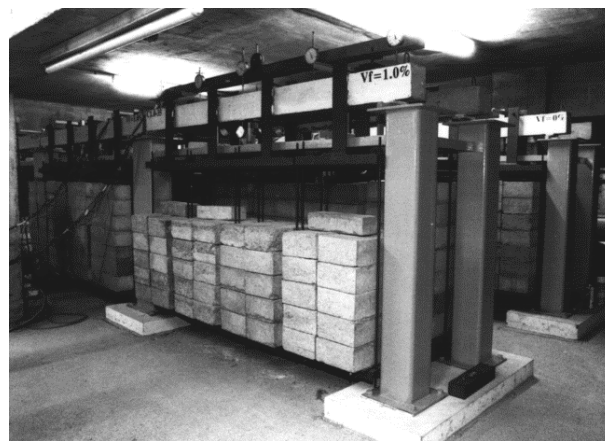
Figure 8. Experimental setup for testing FRC beams (authorized reprint from [98]).
