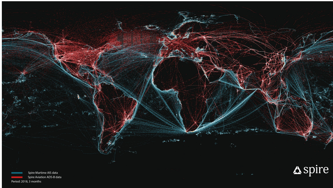
Figure 4.8: Global AIS and ADS-B data after 3 operational months. Image Credit: Spire Global Inc. [202].
