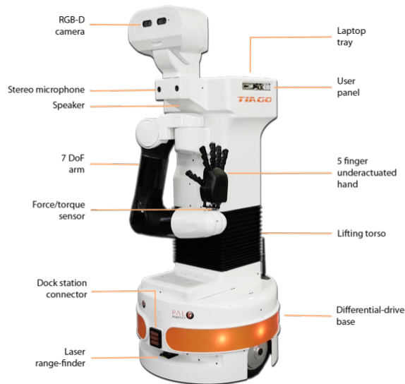
Figure 1.3: The TIAGo robot.
