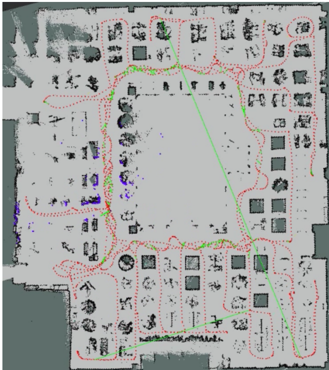
Figure 3.8: Occupancy grid of a large mall floor (approx. 2900m^2 ). Red dots represent robot key frames and green edges loop-closures. During mapping, 415 loop closures were detected of which only 2 were false positives, easily eliminated using distance constraints.
