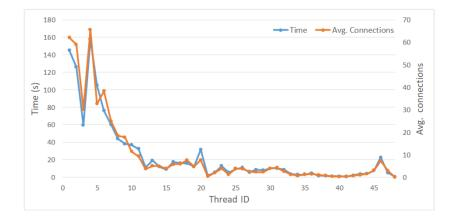
Fig. 3: Correlation between the average number of connections per element and the useful execution time per thread ID.
