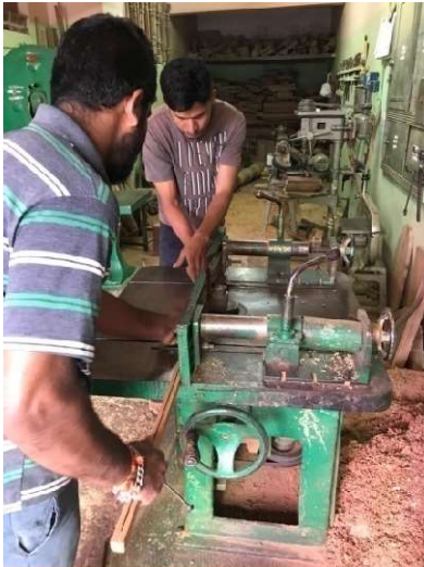
Figure 8 Local artisans manufacturing the wooden dowels
