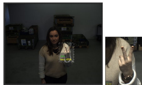
Figure 4.12: Selected ROI and identification window of Classification ANN in the Location + Classification structure
