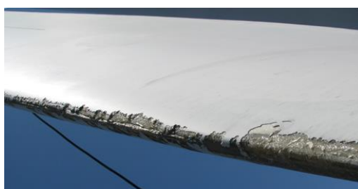
Figure 1. Leading edge erosion [3]
