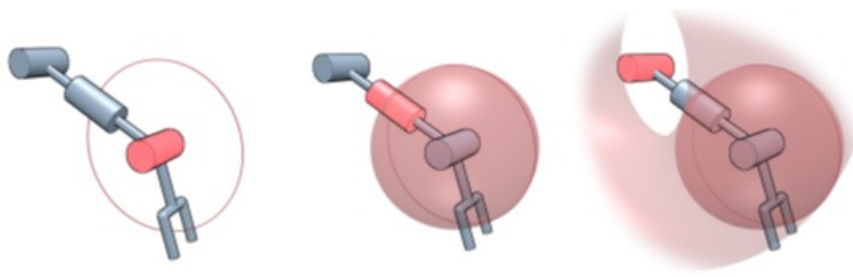
Figure 3.4: Volume sweeping example for the last three joints of a spacial manipulator. Source: [22].
