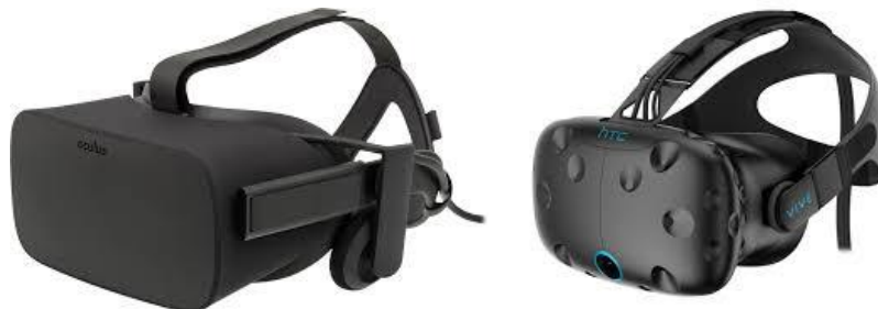
Figure 3.4. Oculus Rift HMD (15) on the left and HTC Vive HMD on the right (16)
