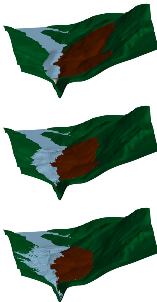
Fig. 20 Example of landslide-water interaction modelled with the PFEM (the Vajont landslide). Pictures from [30]
