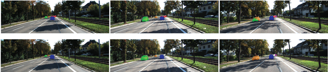
Fig. 1. Qualitative results on three non-consecutive frames comparing the baseline model (row 1) and the model with best performance: inverse step (row 2). Compared to the inverse step strategy, during all the sequence, on the baseline model a wrong mask in red is observed next to the blue instance. Also, the orange mask is confused by the green mask.
