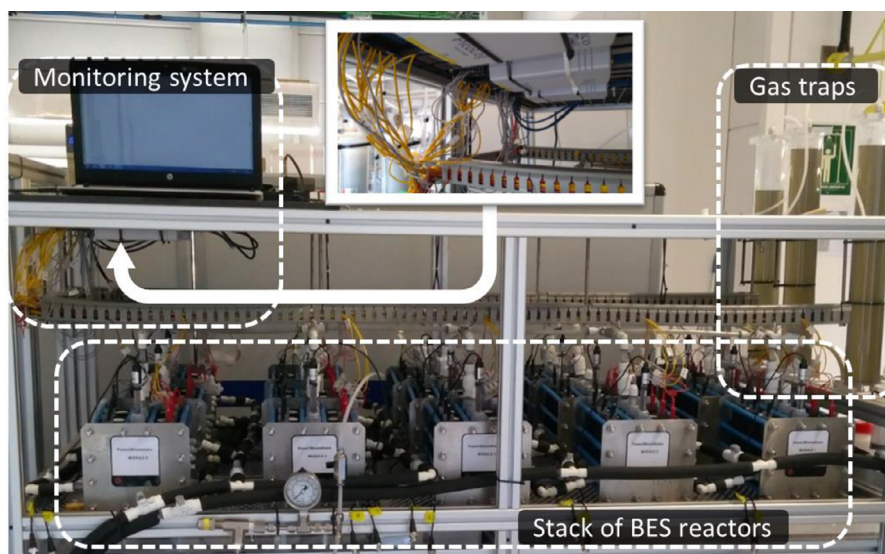
Fig. 2. Stack of reactor modules composing the EMG-BES prototype.
