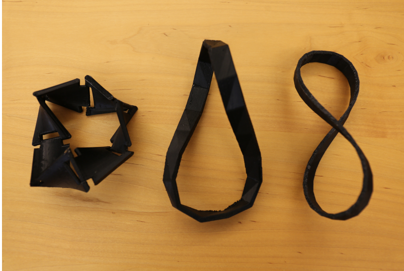
Figure 5: 3D-printed Bernoulli kaleidocycles with 7, 17 and 31 links. The 7-link one has actual hinges and can be everted, but the other ones have been 3D-printed into a particular configuration and do not have hinges because of technical limitations. As N grows, the linkages tend towards a planar lemniscate. The shown objects were designed and printed by Michael Grunwald.
