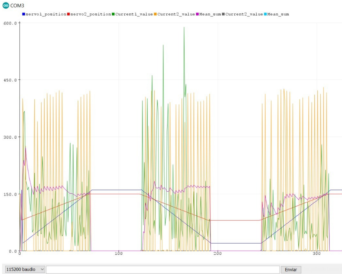
Figure 37: Servo’s current consumption without load.
