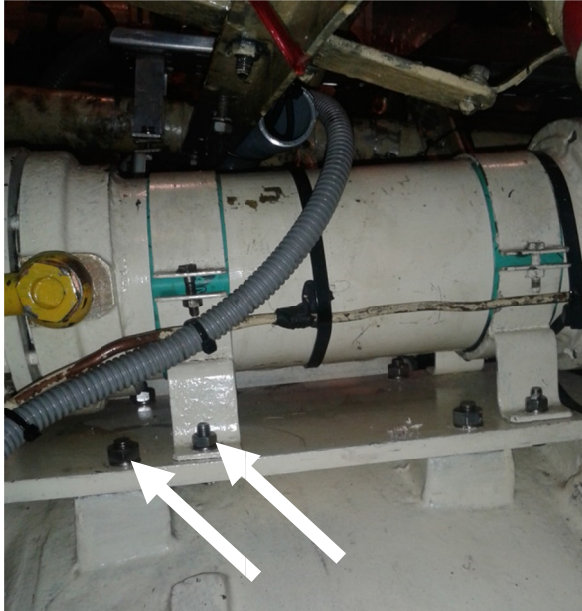
Figure 10: Rigid mounting oil pump (b) and heat exchanger (a) [6]
