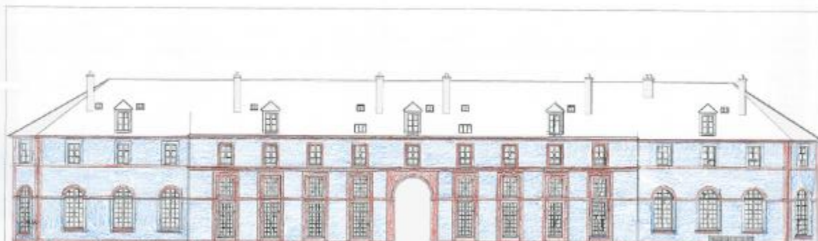
Figure 33- Marking of stones and plasters according to the facades (stones in red and coated in blue)
