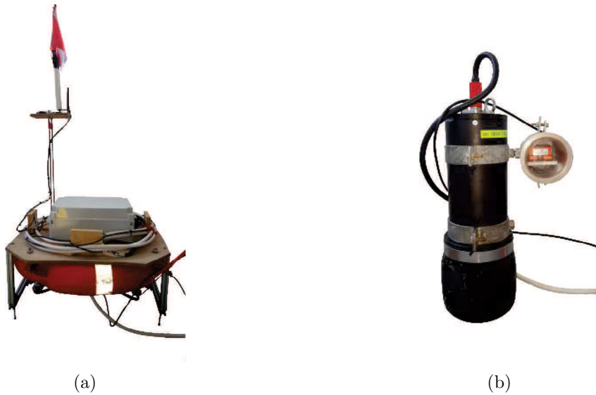
Figure 1: The buoy used to locate the underwater target (Figure 1a) and the IMU-USBL subsystem (Figure 1b).
