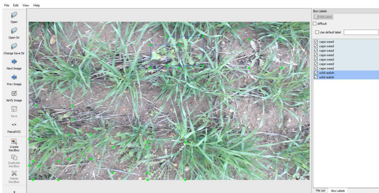
Figure 4. A Labelling tool to label plant images under practical field conditions with multiple bounding boxes.
