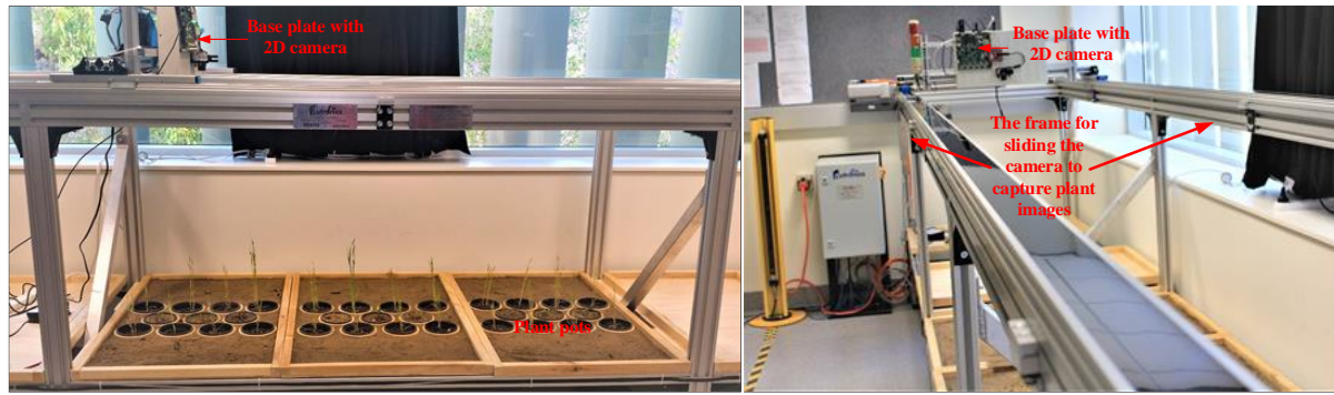
A Testbed system used to capture plant images in the laboratory
