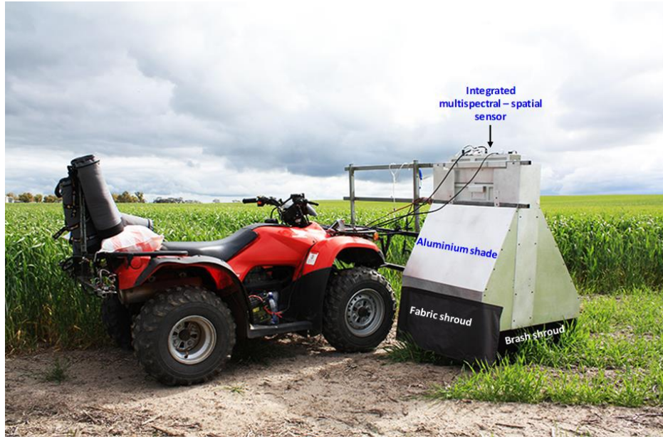
Figure 8. An integrated weed sensing system with the combination of multispectral and spatial sensors in the field.
