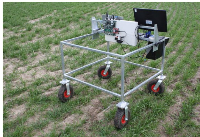
Figure 7. A weed sensing trolley with a Zynq ZC702 development board
