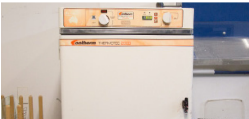
Figure 22. Contherm Thermotech 2000 oven for drying materials
