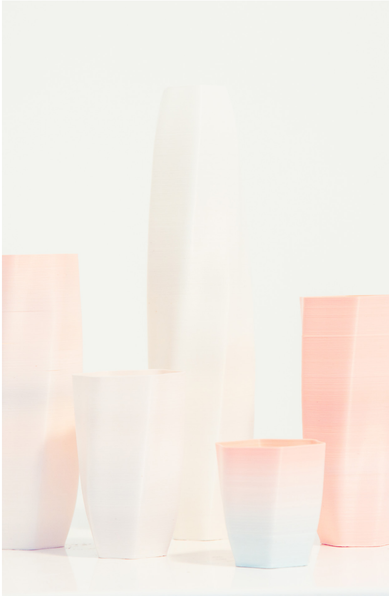
Figure 50. 3D printed with a 100% recycled used PLA HDPE and PP
