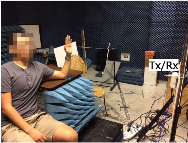
Fig. 2. Measurement setup and a participant seated in an anechoic chamber.
