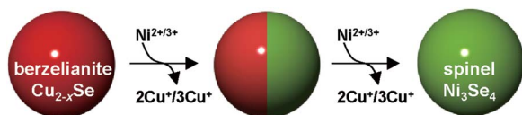
Scheme 1 Schematic of the cation exchange reaction of ber-Cu 2–x Se NCs with Ni cations.
