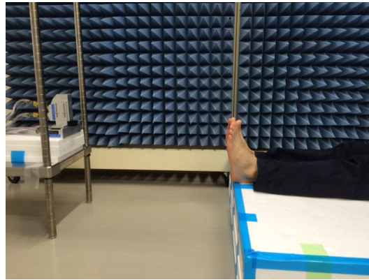
Fig. 2. Measurement setup using 60-GHz radar with a subject in the supine position on a Styrofoam board.
