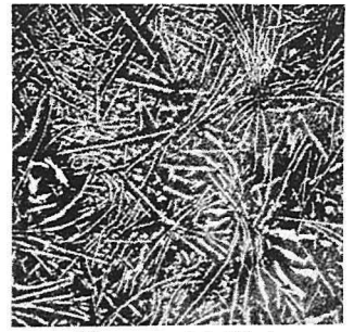
Photo 3. Modified with 0.3% Na \times 100
