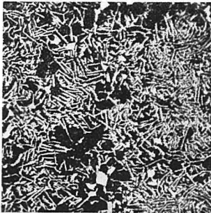
Photo 21. Modified with 0.15% As \times 100
