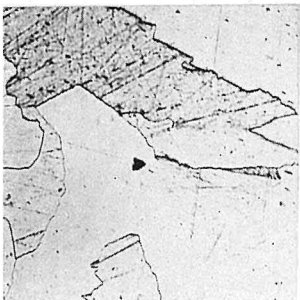
Photo 1. 7.0% Al Quenched from 750°C in ice-water.
