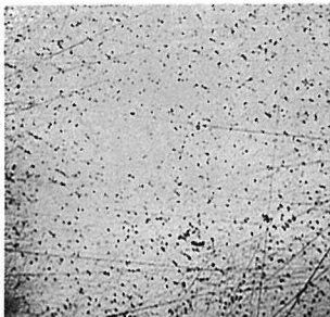
Photo 4. 7.0% Al Quenched from 670°C in ice-water.
