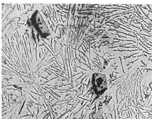
Fig. 14.—Modified with 4.5% Bi. \times 100
