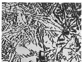
Fig. 15.—Modified with 0.5% Sb. \times 100
