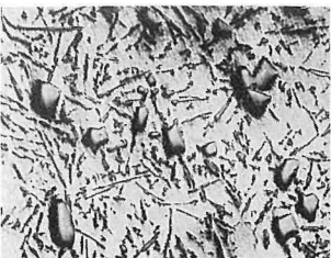
Fig. 13.—Modified with 0.1% Bi. \times 100
