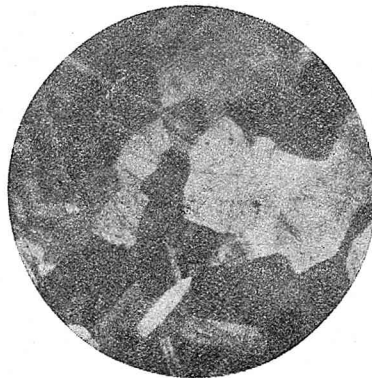
No. 46. Copper-zinc alloy, containing 30 % Zn, annealed for 3 hours at 650. o
