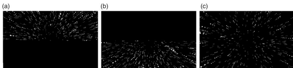
Figure 1. Optic flows generated on the displays by the moving viewpoint. Spheres are distributed within (a) upper, (b) lower, or (c) full area of the VR scene. Note that the actual visual stimuli were viewed with binocular disparities.
