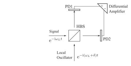
Figure A1. Simple schematic illustration of the heterodyne configuration.
