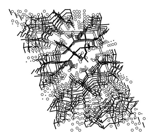
Fig. 4 Perspective view of the  $\text{Li}_2(\text{EMIm})(N(SO_2CF_3)_2)_3$  structure from the b-axis. Large circles denote fluorine atoms. Li-O bonds are drawn in solid lines and H atoms are omitted for clarity.
