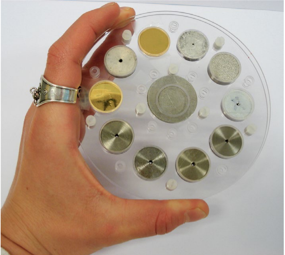
Figure 29. A neutron detector based on 11 different metal discs.
