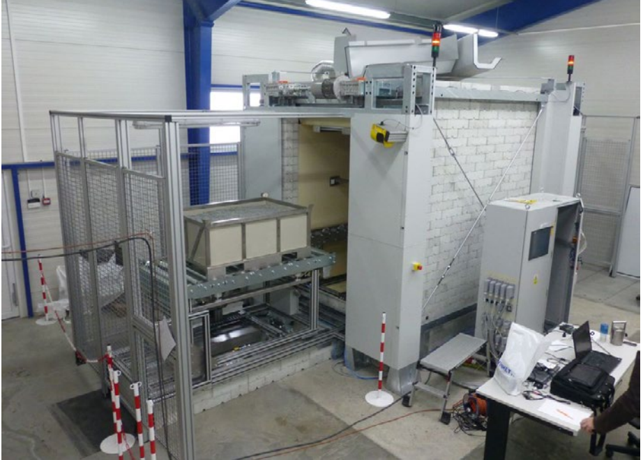
NB: The facility was developed by the Czech Metrology Institute and Envinet within the EURAMET (EMRP) (17) project Metrology for Radioactive waste Management, in which JRC was a partner. Photo: Mikael Hult.
