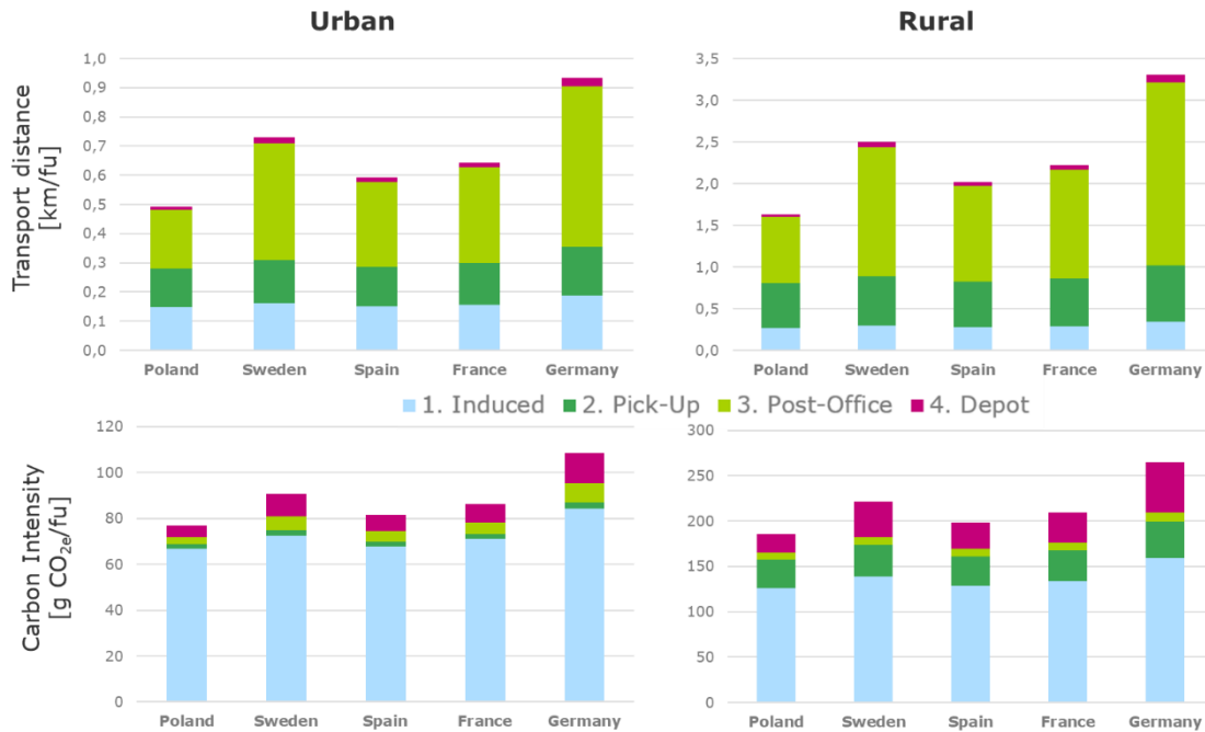
Figure 14: Results for the induced parcel transport and Carbon Dioxide Intensity per fulfilled unit (fu)
