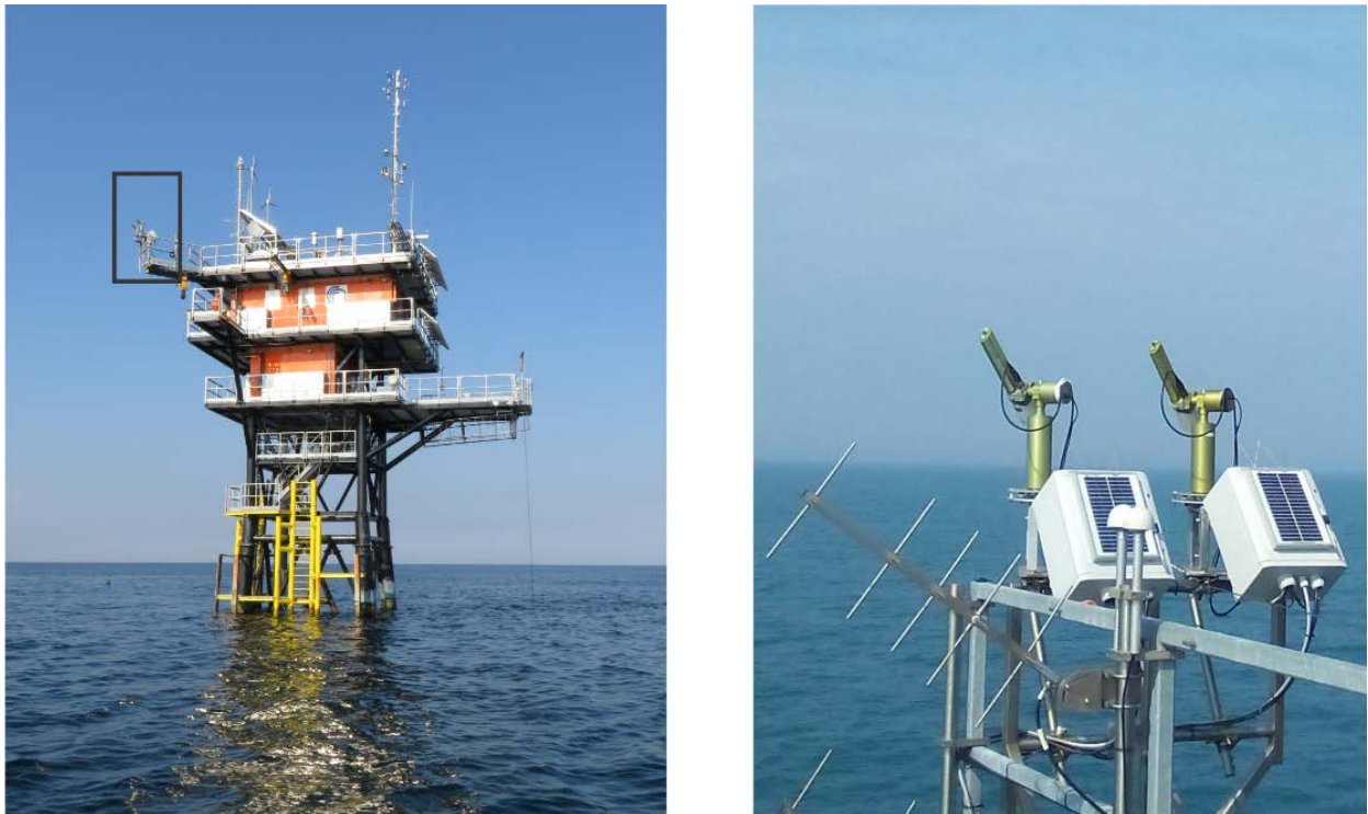
Figure 23. AAOT ( left panel ) and detail of the deployment jetty ( right side ) hosting the CE-318 and CE-318T collocated radiometer systems operated to verify the equivalence of their performance (after Zibordi et al. 2020).
