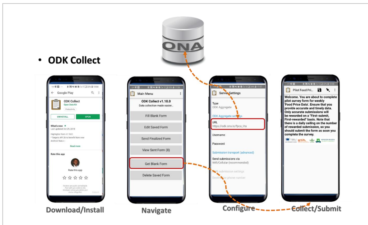
Figure 5. User interface steps for FP CA data collection using the smartphone-based ODK app
