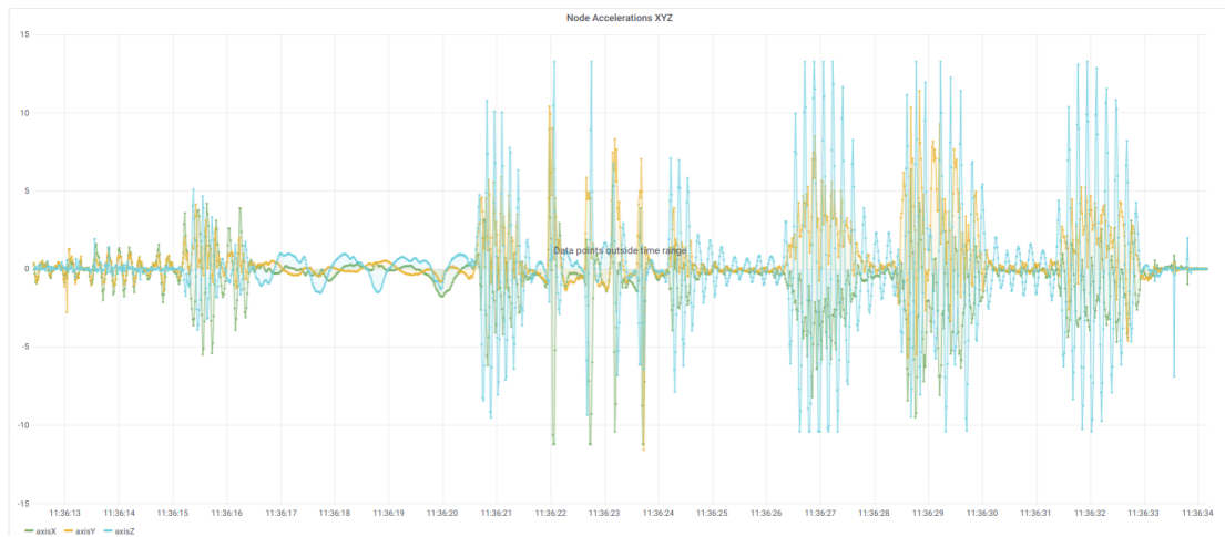
Figure 9: Multiple axes details visualization of accelerometer wireless node.
