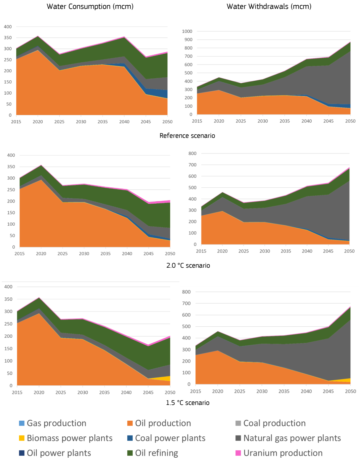
Figure 1. WAPP water consumption and withdrawals by fuel type for the three scenarios
