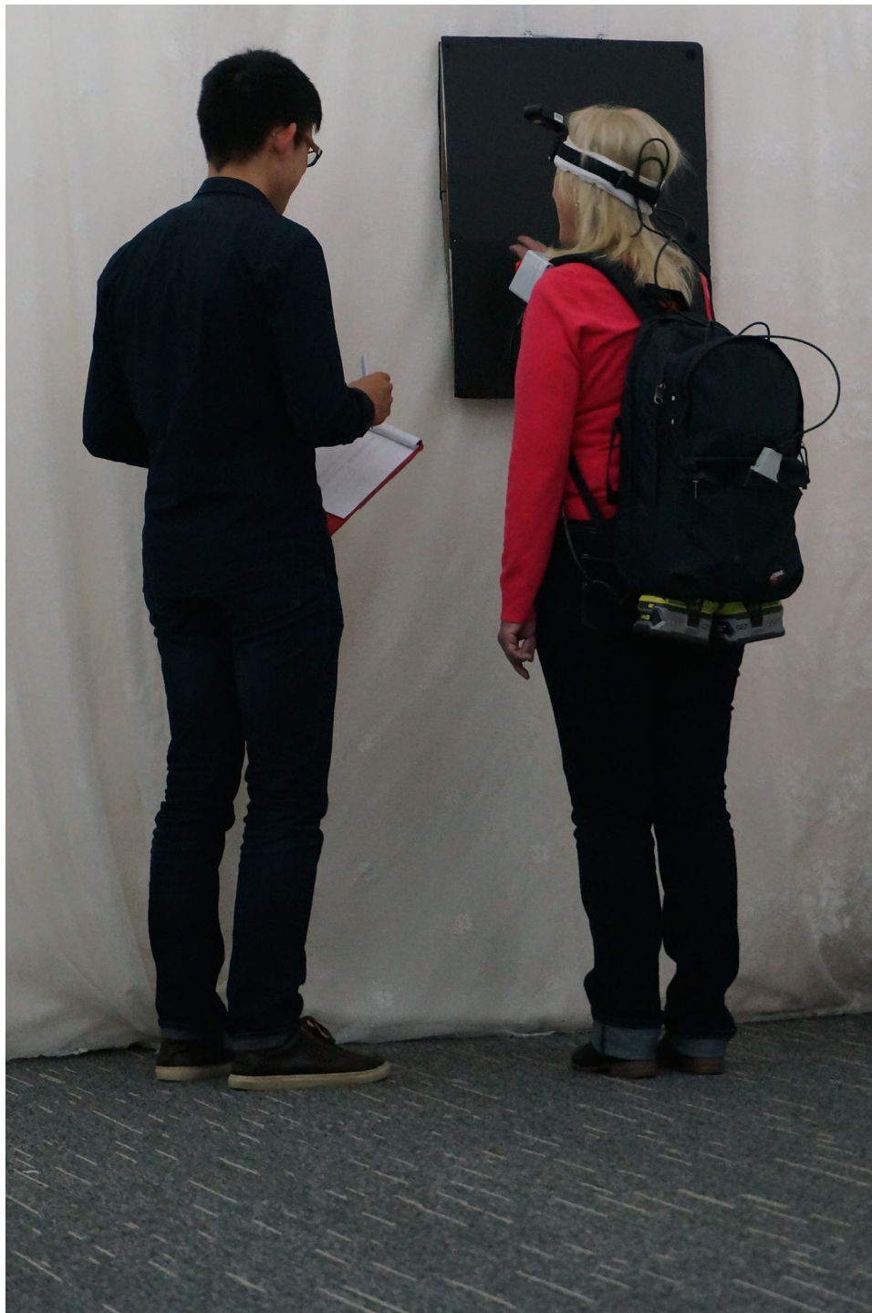
Figure 10. Example of the “find the door” task, used by research groups including Second Sight (USA) and Bionic Vision Technologies (Australia) as an orientation task. Image courtesy of the Centre for Eye Research Australia and Bionic Vision Technologies (Australia).
