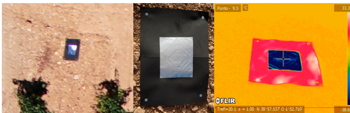
Figure 6. Type of GCPs used in thermal images.
