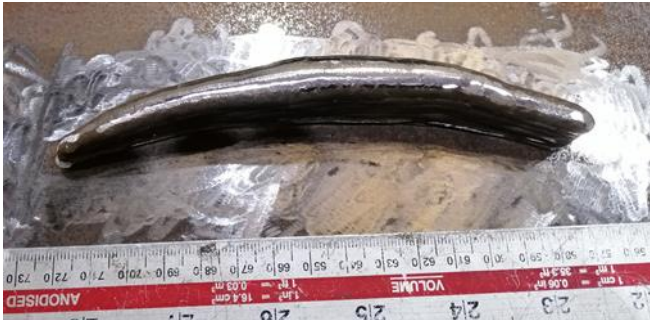
Figure 16 Wall of variable width deposited by MFAILC controller
