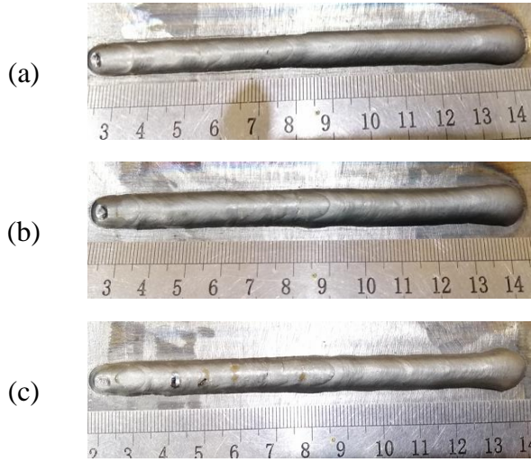
Figure 14 Appearances of weld beads in robustness experiments (a). 1h iteration (b). 2th iteration (c). 3th iteration
