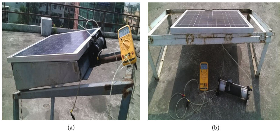
FIGURE 4: Digital multimeter is connected to measure the voltage and current. (a) The PVT system and (b) the normal system.
